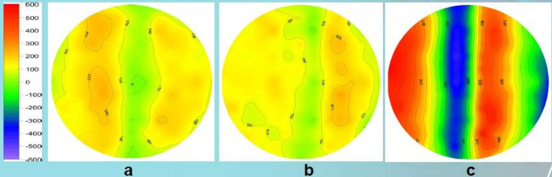
Two dimensional residual stress mapping through the interior of a 14 mm coil rod showing the stress components from the internal bore (left) to the external diameter: (a), Hoop; (b), Radial (along spring length); and (c), Axial (along the coil). The neutron strain scanning was done with a gauge volume of 1 mm<sup>3</sup>.
